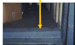
**i** You should not need to step up from edge of container to get inside; there should be no steps or raised platforms inside container.
