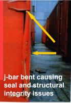
Cargo container doors should seal completely and securely when shut. The container should be light-tight, which will also prevent entry of any external elements into the container while in transit. To ensure a satisfactory light-tight seal, you can conduct a light test by observing the seal performance from inside a closed container. In addition, all door locking hardware (hasps, hinges, handles, bars, bolts, etc.) must be tested and be in good working order (see below diagram).
